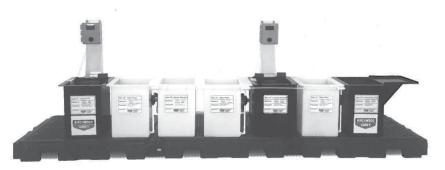
B&B Manufacturing has invested in a new Low Temperature Black Oxide line from Birchwood Casey. This system brings a previously outsourced process into B&B Manufacturing allowing us a cost-effective solution with a quicker turn around time. This particular system named TRU TEMP® provides a finish without Salt Bleed Out on all non-Stainless Steels and Cast Iron while remaining safe, operator friendly, RoHS compliant, and with no EPA problems.
